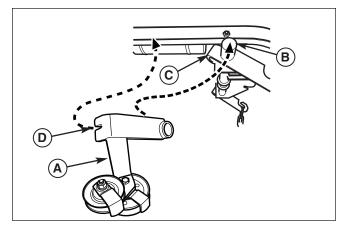
Figure 8. Front Idler Pulley Installation
